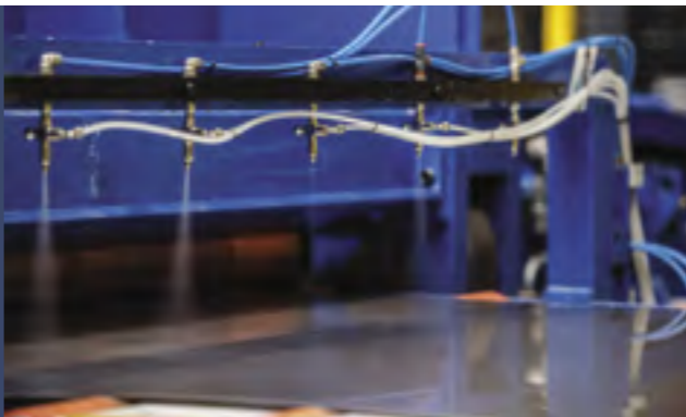
Cleaning of Strip and Rolls for Levelling Cassette
