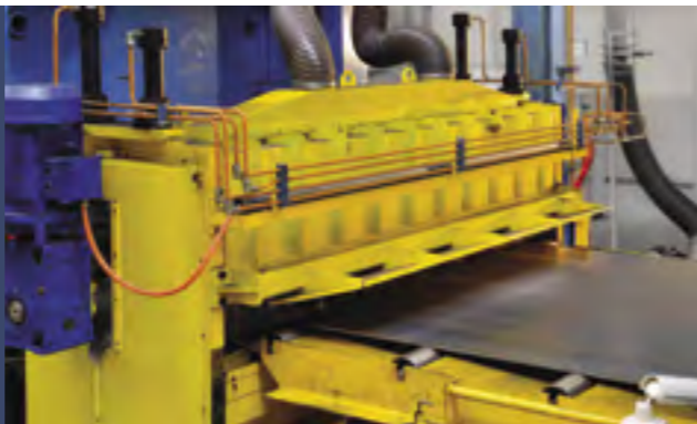
Multiple Brushing System for Scale Removal
