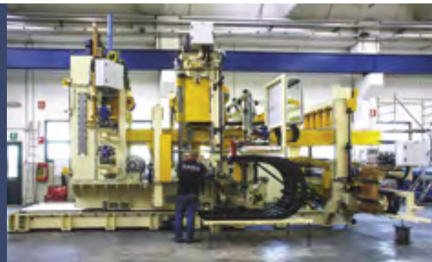
Slits Threading Grippers from Slitting Shear to Recoiler Mandrel
